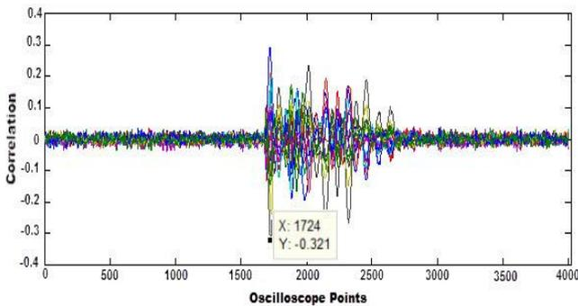
Fig. 9. EM attack correlations using the HW model.
