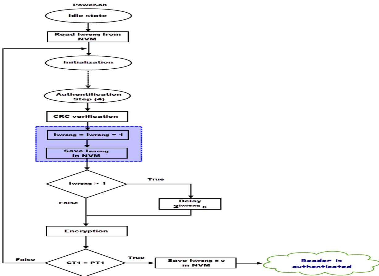
Fig. 11. State diagram describing the countermeasure at ProtocolS.
