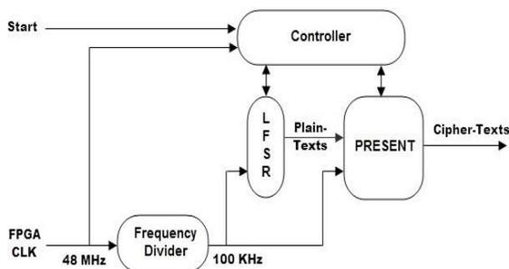
Fig. 6. Design architecture controlling the PRESENT block cipher during EMA.
